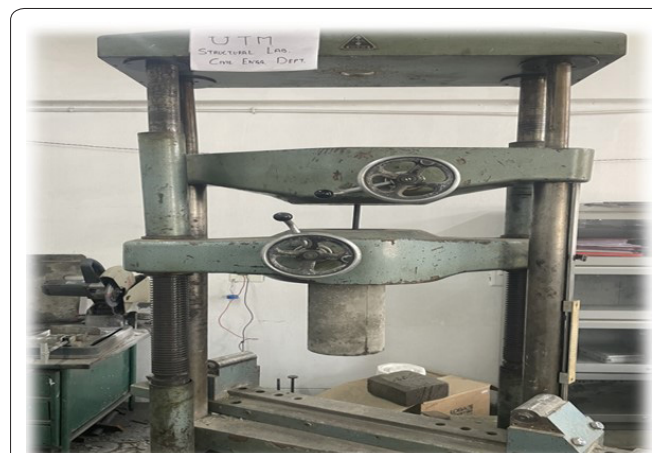
Figure 2: The setup for the tension pullout test.
