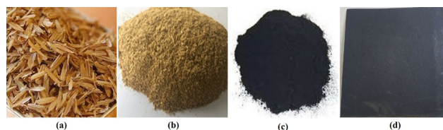
Figure 1: (a) Raw RH, (b) RH powder after treated with H_2O_2 , (c) GO, and (d) Fabricated RH and GO particle board.
