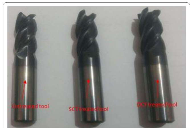
Figure 2: WC cutting tools utilized.
