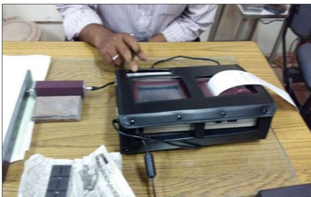
Figure 6: Surface roughness measurement.
