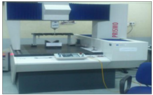
Figure 5: Hole geometry measurement using CMM.
