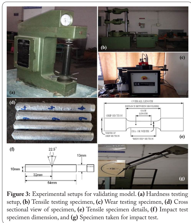
Figure 3: Experimental setups for validating model. (a) Hardness testing setup, (b) Tensile testing specimen, (c) Wear testing specimen, (d) Cross sectional view of specimen, (e) Tensile specimen details, (f) Impact test specimen dimension, and (g) Specimen taken for impact test.
