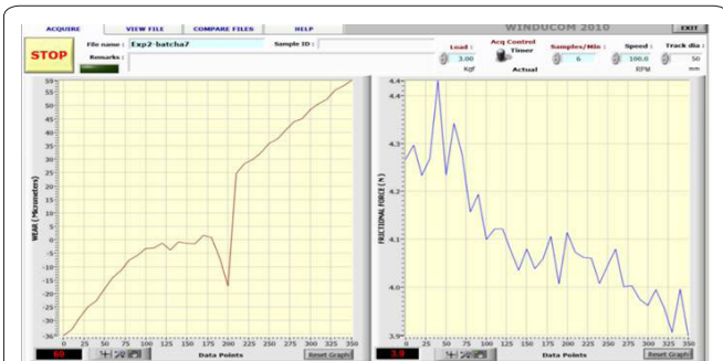
Figure 5: Variation of wear, frictional force, and COF in relation to time (Soybean oil + aluminum pin, load - 30 N, Speed - 100 rpm, and time 360 s).
