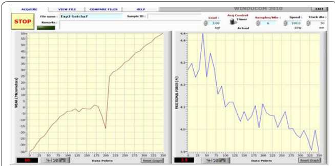
Figure 4: Variation of wear in relation to time (Soybean oil + aluminum pin, load - 30 N, Speed - 100 rpm, and time 360 s).
