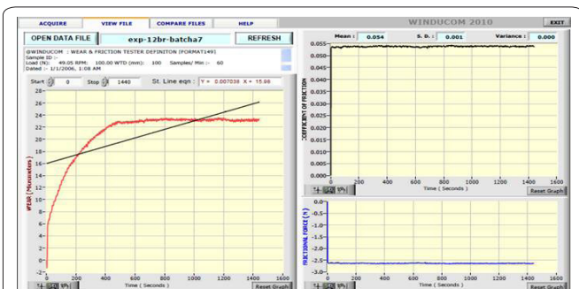
Figure 6: Variation of wear in relation to time (Soybean oil + brass pin, load - 50 N, Speed - 300 rpm, and time 1440 s).
