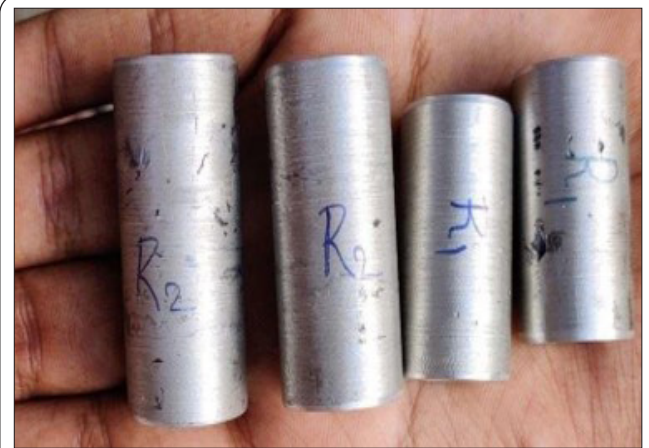
Figure 11: Compression pieces before testing.
