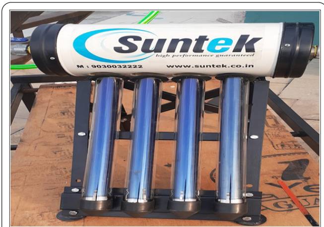
Figure 2: Evacuated tubes used in the experimental setup.
