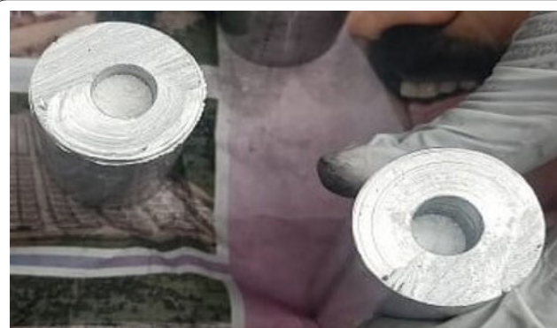
Figure 2: Feeding nano kaolinite to novel encapsulated AA5059.
