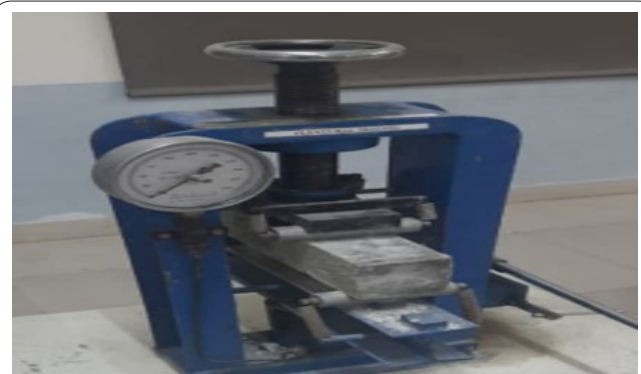
Figure 3: The data on flexural strength were collected using a tensile testing machine.
