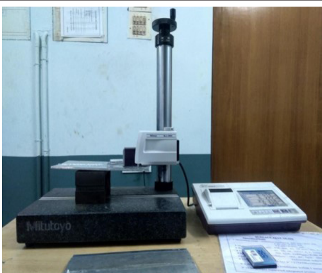
Figure 4: Mitutoyo-SJ-410 surface roughness tester while testing the samples.
