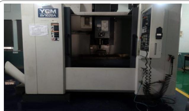
Figure 2: Vertical Milling Machine for machining a slot in the aluminum composites (AA6063/SiC/TiO 2 ) HMMCs using HSS and carbide tool.
