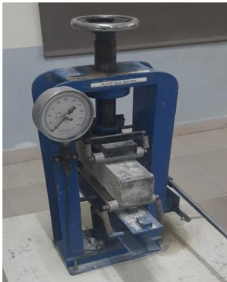
Figure 4: Flexural strength testing machine.
