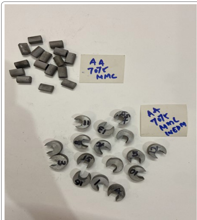
Figure 2: Al7075/5%B 4 C + 2% Mg after wire electric discharge machining.
