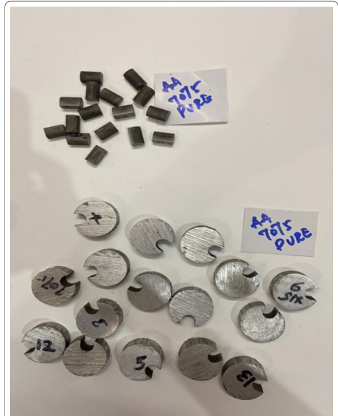
Figure 1: AA7075 pure alloy after wiring electric discharge machining.
