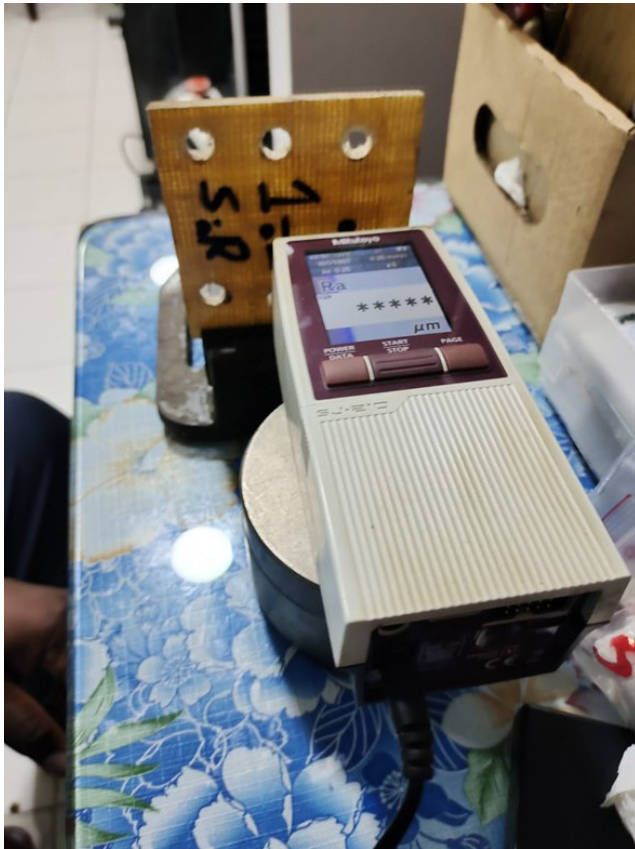
Figure 2: Surface testing loading of the specimen.
