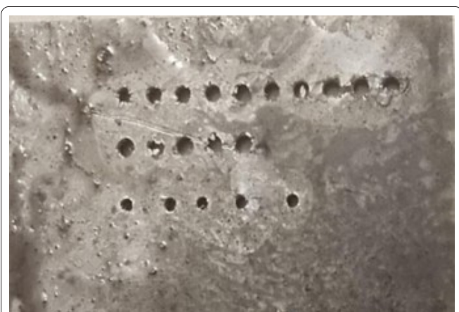
Figure 2: CNC drilling on novel hybrid reinforced epoxy (Group 1).
