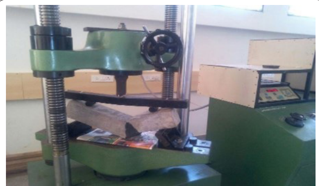
Figure 3: Testing of beam specimen.
