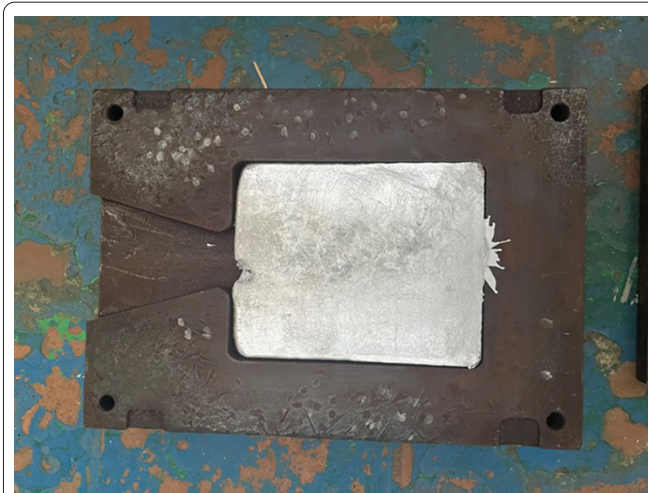
Figure 3: Casting of aluminum metal composite without SiC reinforcement.
