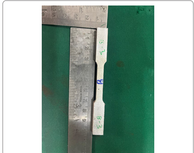
Figure 4: Tensile sample specimen as per ASTM standard machined by CNC machining.
