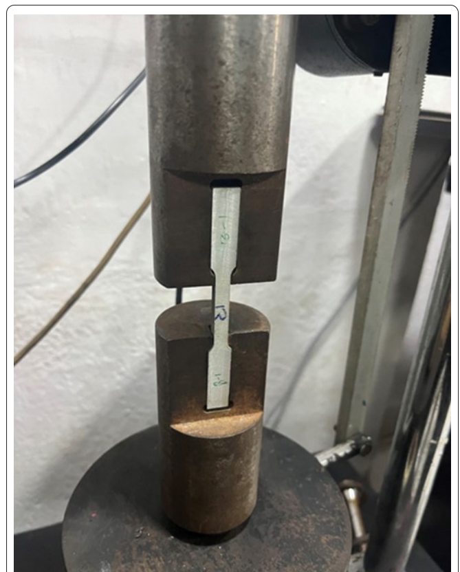
Figure 5: Tensile testing of the aluminum alloy AA5083 base material.
