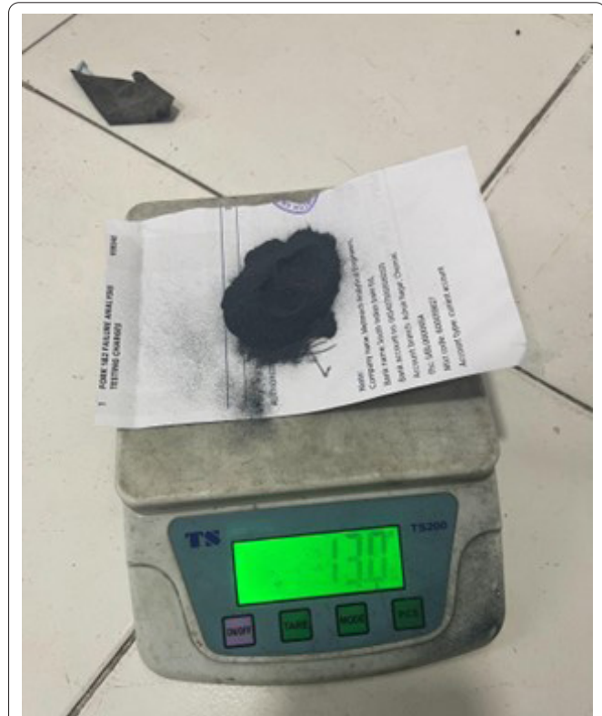
Figure 2: SiC particulate material used for casting process.
