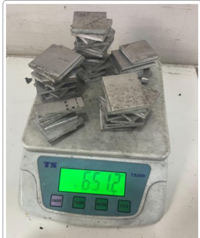
Figure 1: Aluminum AA5083 metal used for casting of base metal.
