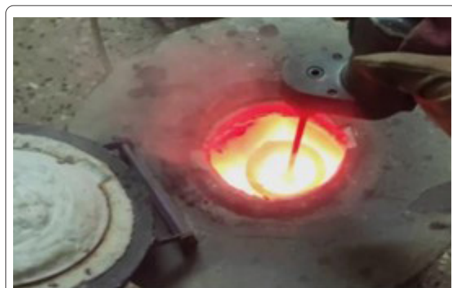
Figure 1: Stir casting process.
