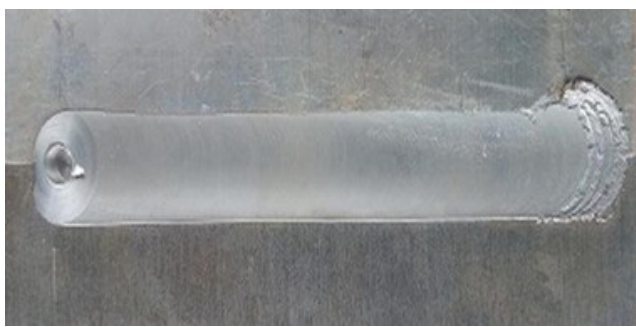
Figure 4: Friction welded joint for rotational speed 1200 rpm, translation speed 60 mm/min, and axial load 10 kN.
