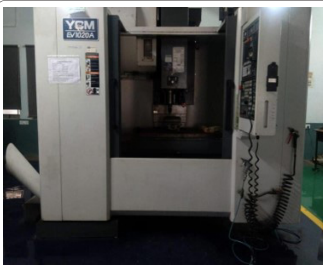
Figure 5: Vertical milling machine for machining for FSW.
