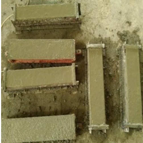
Figure 4: Casting of flexural beams.
