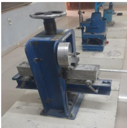
Figure 5: Flexural strength testing arrangements.
