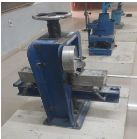
Figure 5: Flexural strength testing arrangements.
