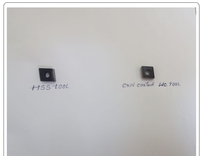
Figure 3: HSS tool and CrN coated WC tool.
