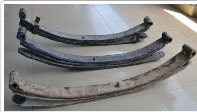
Figure 1: Fabricated composite leaf springs.
