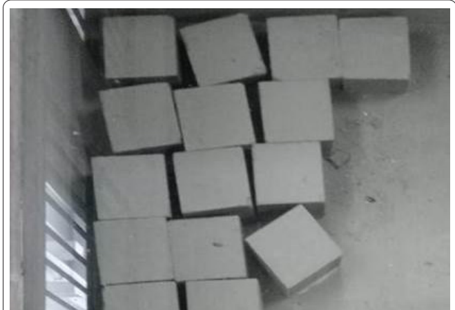
Figure 5: The concrete cube was placed in the curing ponds at the period of 28 days.
