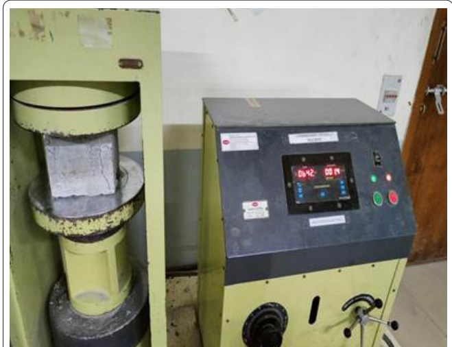
Figure 4: Compressive strength test for concrete cube.
