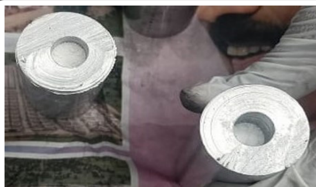
Figure 2: Feeding nano \text{Si}_3\text{N}_4 to novel encapsulated AA4032.
