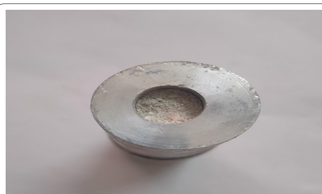
Figure 2: Feeding of 5% fly ash and 5% nano ZrO 2 to novel encapsulated AA7178.
