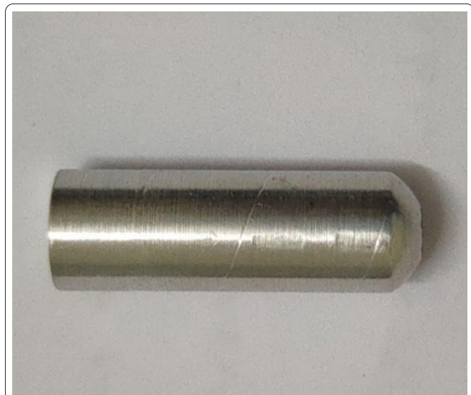
Figure 6: Reinforced specimen after wear testing.
