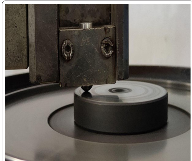
Figure 5: Specimen is undergoing wear test on the counter surface of pin-on-disc equipment.
