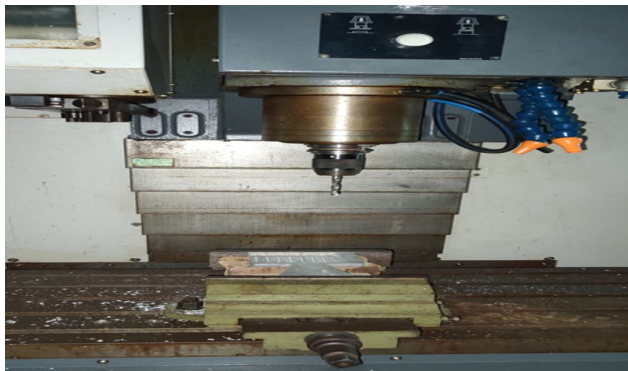
Figure 4: Material is drilled by CNC for surface roughness testing.
