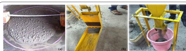
Figure 1: Test arrangement for fresh state properties of SCC mix. (a) Measurement of slump flow, (b) Test arrangement for L-box test, and (c) Test arrangement for V-funnel test.
