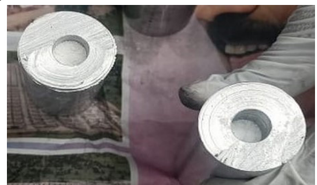
Figure 2: Feeding nano kaolinite to novel encapsulated AA5059.
