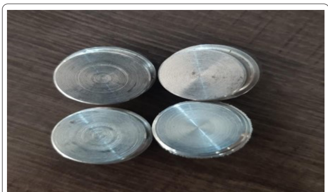
Figure 3: Samples machined using CBN coated.
