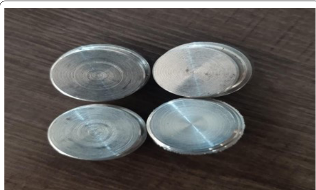
Figure 5: Samples machined using uncoated.
