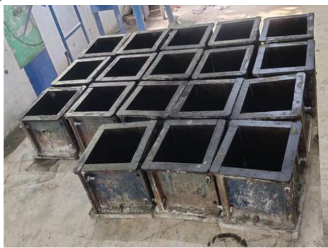
Figure 3: Preparing concrete cube mold.
