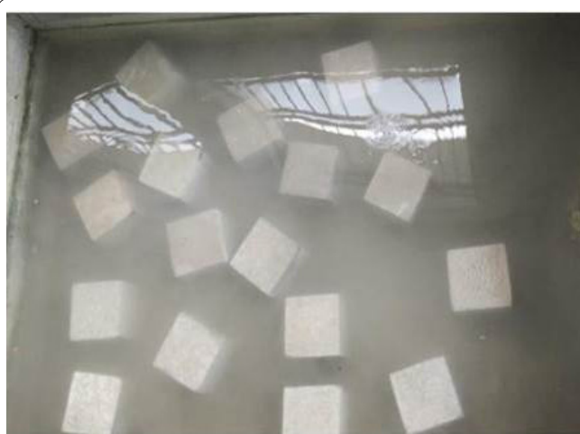
Figure 4: Curing of concrete cubes.
