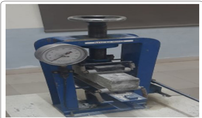
Figure 4: Beam specimen testing by using flexural testing machine.
