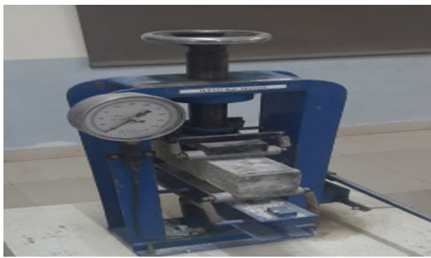
Figure 4: Beam specimen testing by using flexural testing machine.
