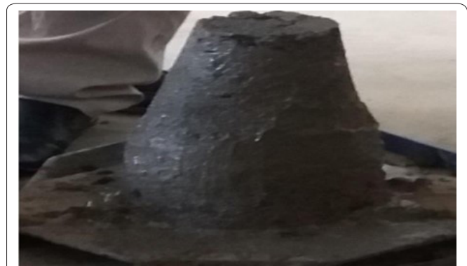
Figure 3: Slump cone test.
