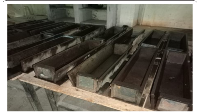
Figure 2: Preparing flexural beam mold.
