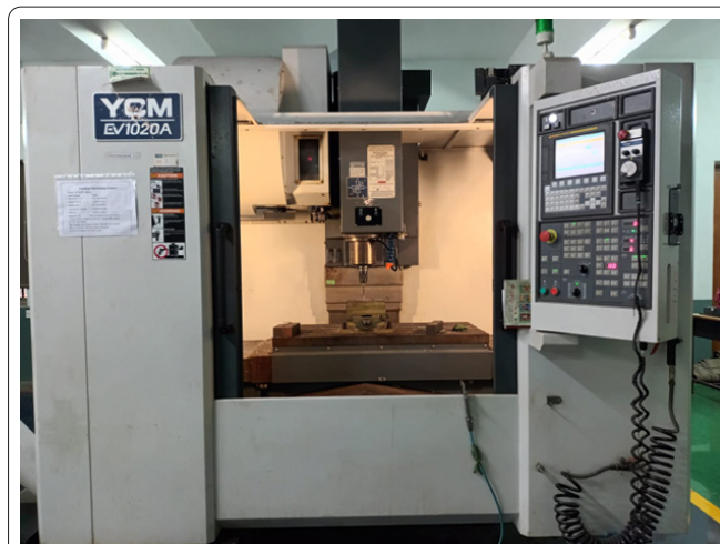
Figure 1: Vertical CNC milling machine YCM XV1020A.
