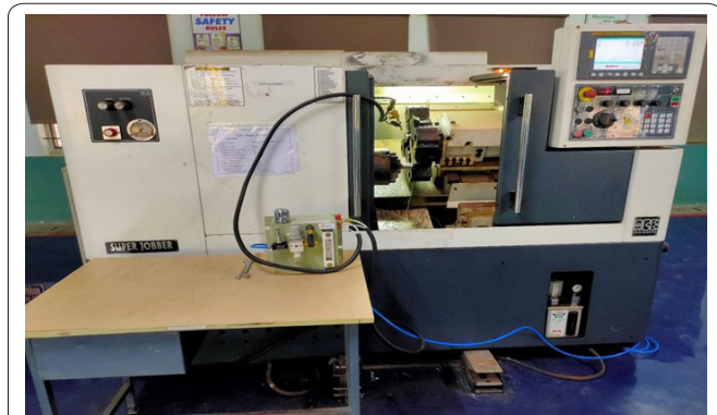
Figure 5: Jobber XL CNC lathe used for the experimental setup; specs include a swing carriage measuring 260 mm, a maximum turning diameter of 290 mm, a maximum turning length of 400/500 mm, a swing bed of 500 mm, a maximum spindle speed of 4000 rpm, eight stations, and a chuck size of 200/250 mm.
