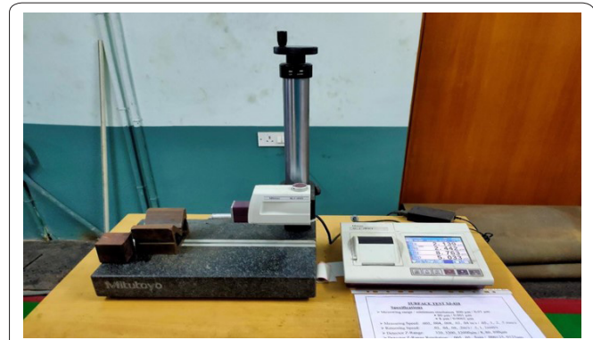
Figure 6: Mitutoyo model SJ-410 surface finish analyzer for surface roughness measurement.
