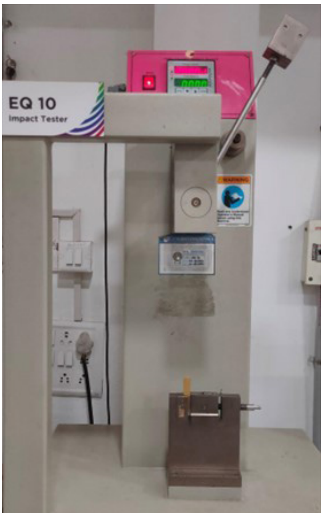
Figure 4: Izod impact strength tester.
