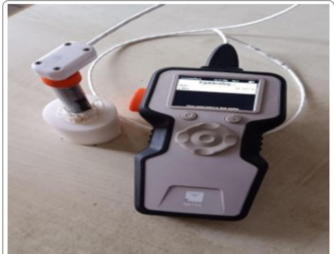
Figure 1: Measurement of thermal conductivity.
