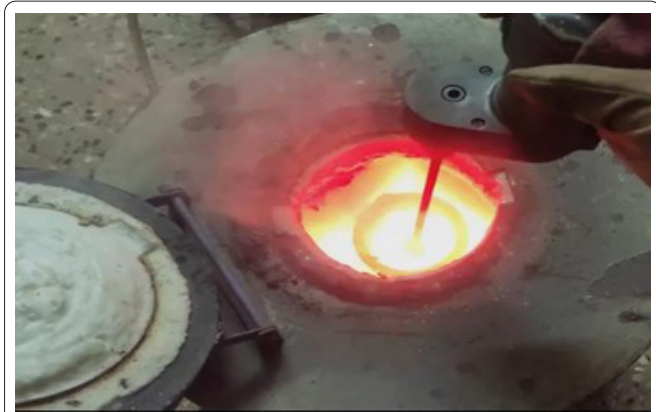
Figure 1: Stir casting process.
