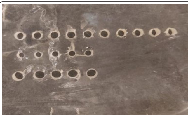
Figure 1: CNC drilling on plain epoxy (Group 2).
