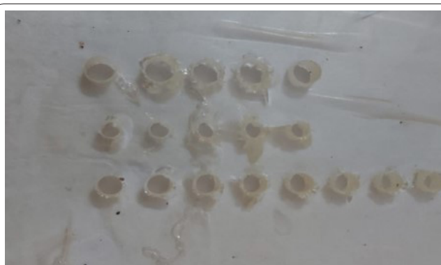
Figure 1: CNC drilling on plain epoxy (Group 2).
