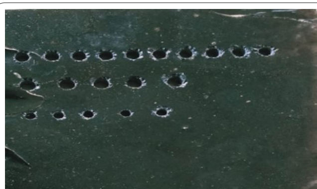
Figure 2: CNC drilling on novel hybrid reinforced epoxy (Group 1).
