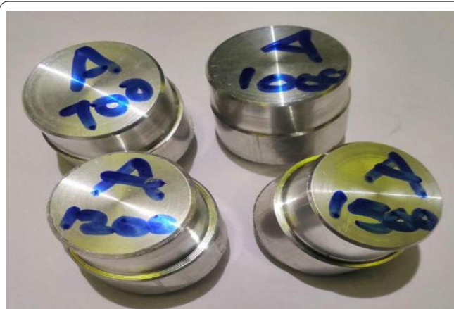
Figure 3: Al-Zn5Mg alloy turned by TiN covered tool.
