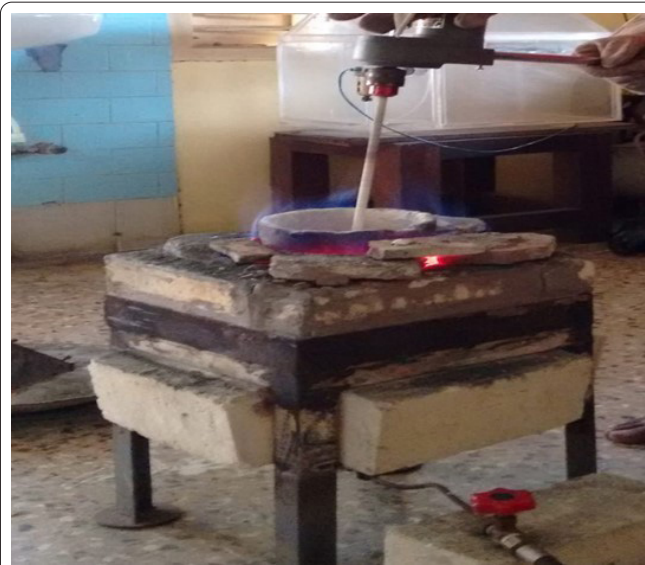
Figure 1: Fabrication setup for the stir casting process.
