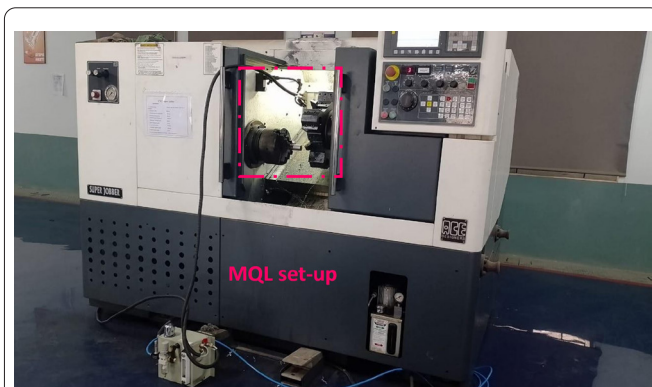
Figure 5: Experimental setup - Jobber XL CNC lathe, specifications: swing carriage - 260 mm, maximum turning diameter - 290 mm, maximum turning length - 400/500 mm, swing bed - 500 mm, max spindle speed - 4000 rpm, number of stations - 8, and chuck size - 200/250.
