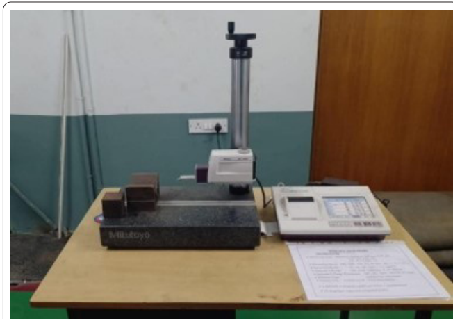
Figure 6: Mitutoyo model SJ-410 surface finish analyzer for surface roughness measurement.
