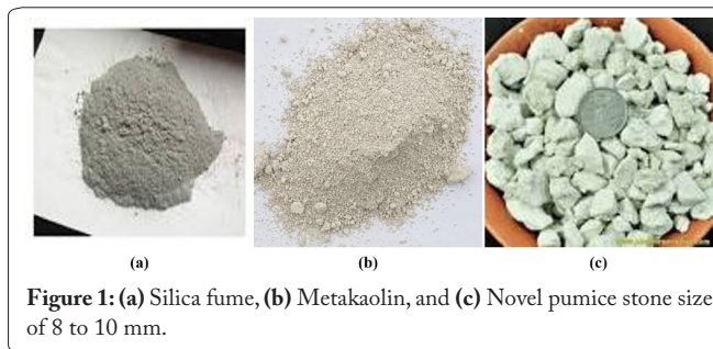
Figure 1: (a) Silica fume, (b) Metakaolin, and (c) Novel pumice stone size of 8 to 10 mm.
