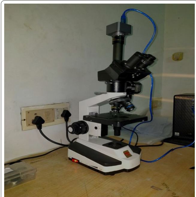
Figure 5: An optical microscope with 10x magnification for flank wear measurement.
