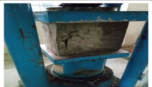
Figure 4: Broken specimen after testing.
