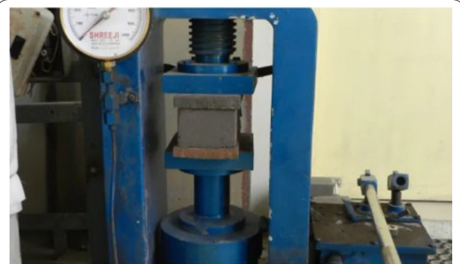
Figure 3: Using a universal testing machine, the compressive strength results were obtained.
