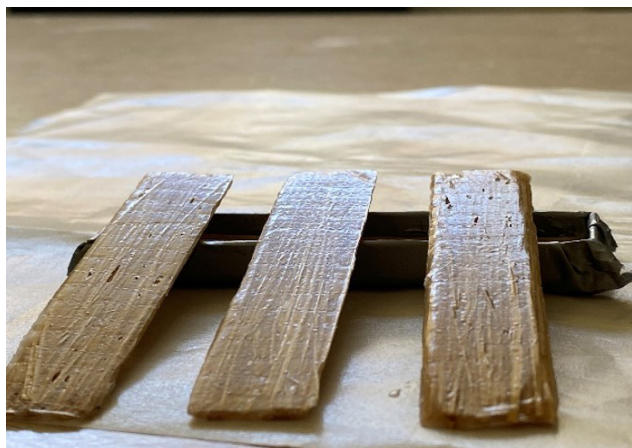
Figure 1: Continuous bamboo fiber composites elaborated using the hand layup technique.
