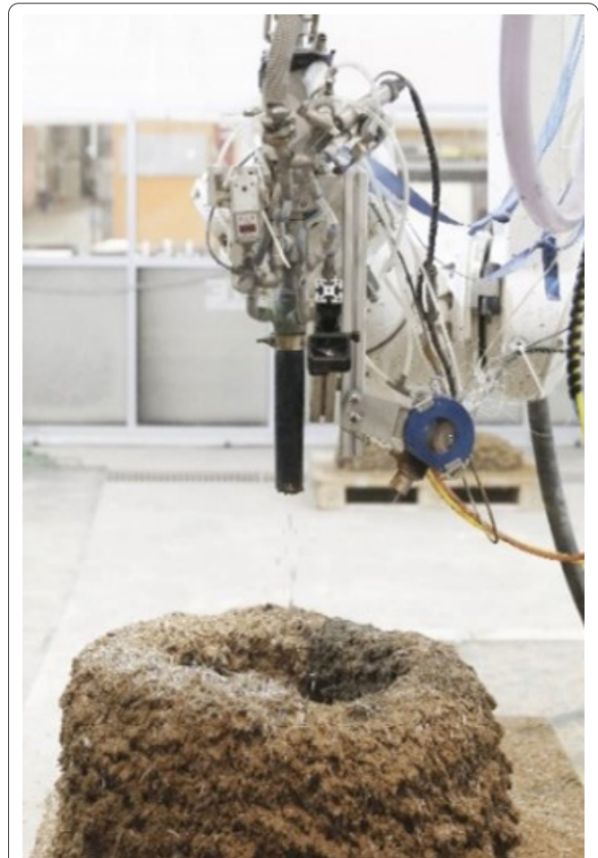
Figure 13: Experimental test setup with fiber chopper pointing at material jet for post-nozzle intermixing of long fibers.
