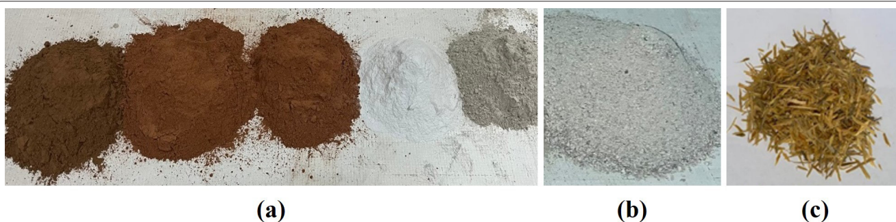
Figure 1: The physical appearance of the CDW-based materials: (a) RCB, HB, RT, G and C from left to right, (b) RCA, and (c) WWFs treated with 2.5 M NaOH for 2 hours.
